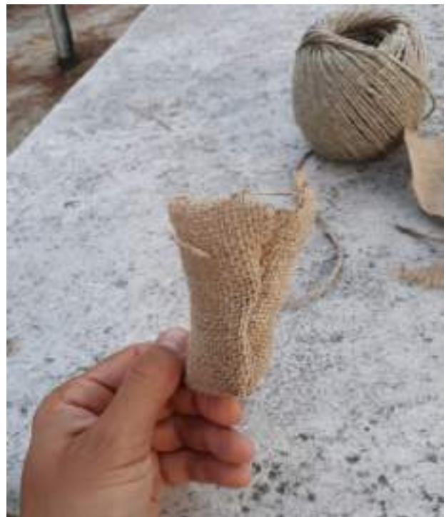
Figure 13. Jute blankets used to place the specimens inside the container (photo by Marco Segarich).
